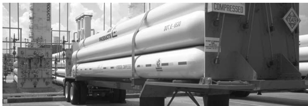
Figure 1 Hydrogen Tube Trailer
