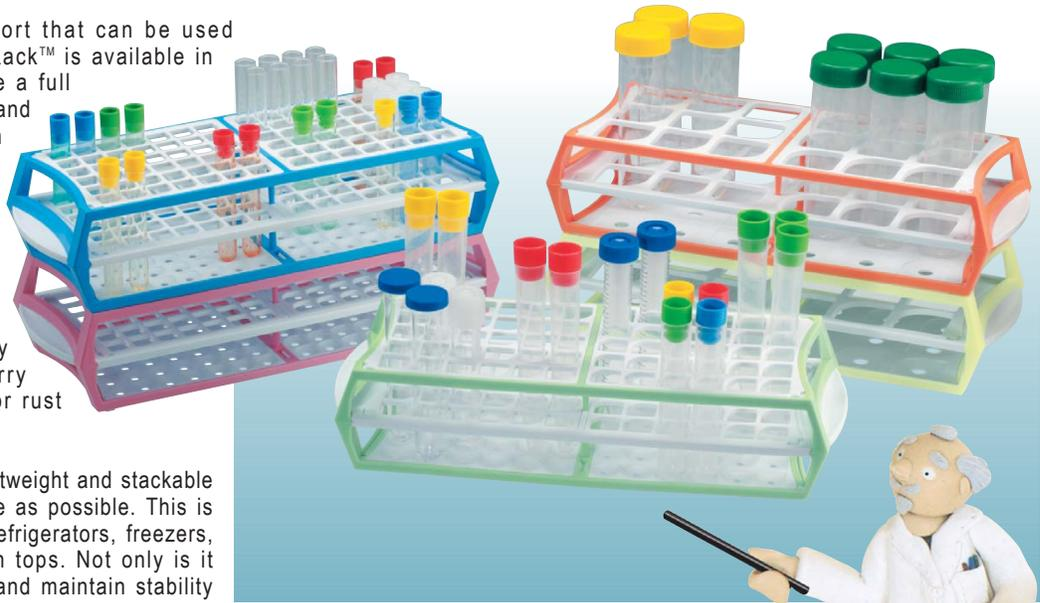
The MultiRack™ is available in 3 models to accommodate a full range of laboratory test tubes and centrifuge tubes up to 30 mm in diameter.
