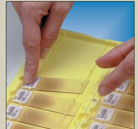
Easy slide removal by pressing down on one end and lifting it from the other.
