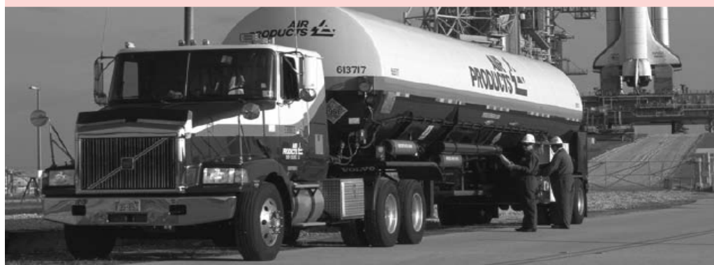
Typical Liquid Hydrogen Tanker
